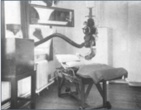
Apparatus for delivering 5g radium source to patient, 1937 Images source: Grimmett LG BJR 1937; 10(110):105-11
