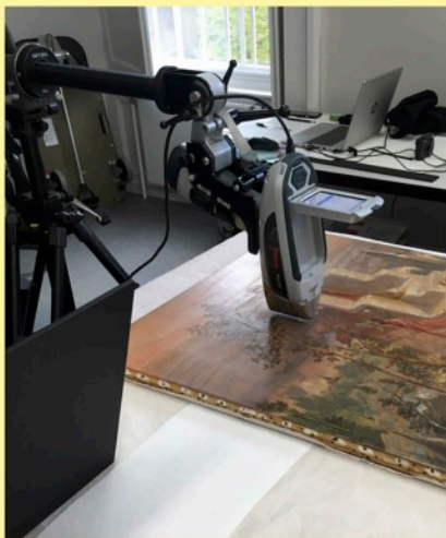
Portable XRF Analyser used for the examination of panel D of The King's Quair by William Bell Scott. 22.Feb.2022
