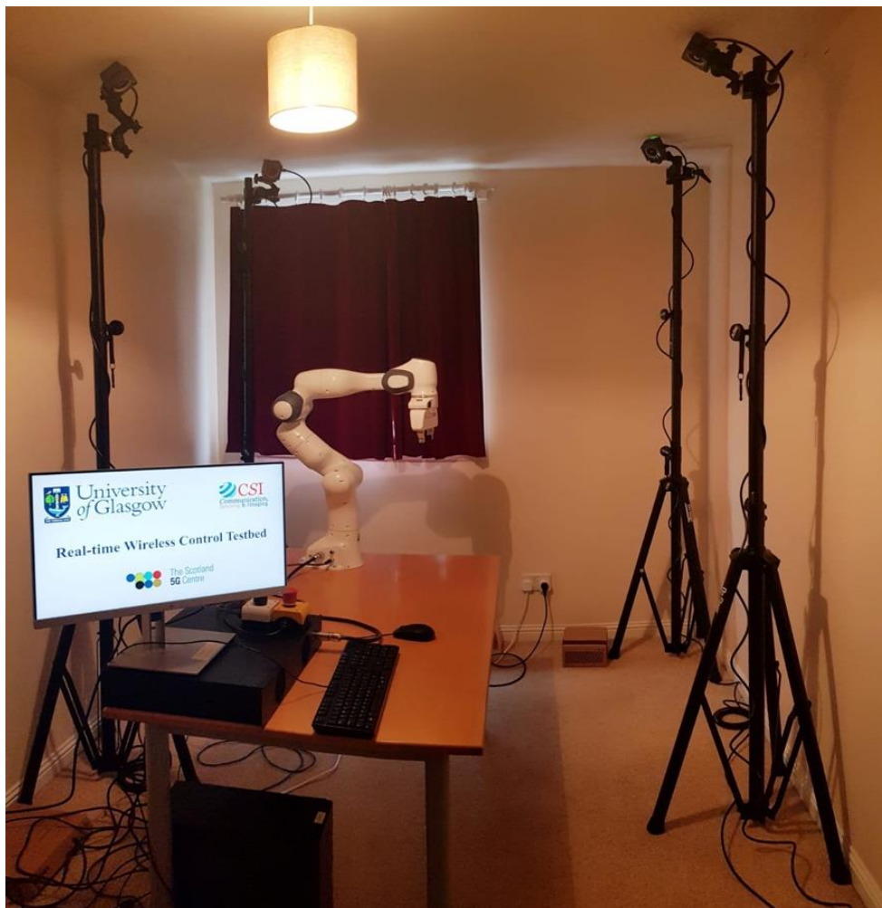
Real-time wireless control testbed with motion capture and robotic arm
