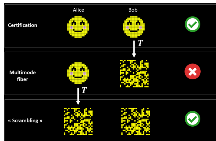
Figure 3. Certification: Alice and Bob certify entanglement by measuring correlated spatial modes of photons (illustrated here by two identical smiley images). Multimode fiber: In the presence of a multimode fiber, the spatial information content of one photon gets mixed and is no longer correlated with that carried by its twin (smiley becomes a speckle). Scrambling: By carefully scrambling spatial information carried by Alice’s photon, it is possible to recover the correlations between spatial information carried by each photon without directly unscrambling the scrambled image (speckles are correlated, but they are not smileys anymore).
