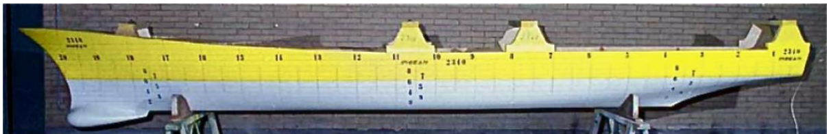
DTMB 5415 Naval Ship Model which I used to test my methodology
