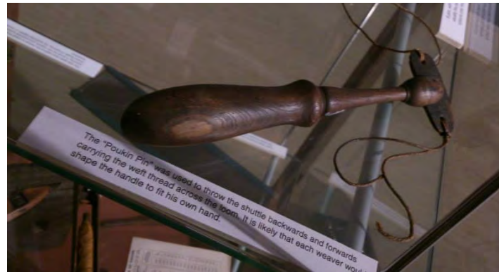
A 'poukin pin' used to throw the shuttle back and forth, in Paisley Museum collec-
