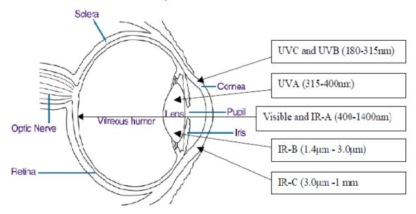
**NB** Short pulsed high peak-power laser beams are particularly hazardous to the eye, especially at wavelengths that reach the retina, as they deliver a lot of energy in a short period of time that can cause irreversible damage. Near infra-red lasers are also particularly hazardous because you can't see the beam but it could be focused on the retina and you would only be aware of it after damage has been caused.
