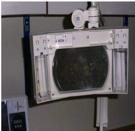
Example of an illuminated magnifier, in this case a Luxo Wave Plus illuminator
