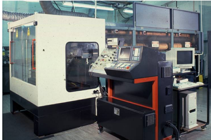
Vision panels in guarded area
